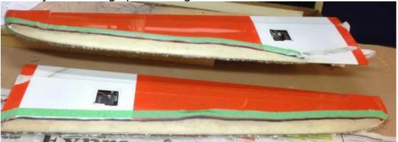
The Superior tip panels have the leading edges filled with foam, shaped then alassed.
